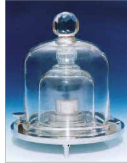
Figure 1: The national standard of the kilogram of the Federal Republic of Germany at the PTB (Braunschweig). It is made of a platinum-iridium alloy and is compared with the international prototype of the kilogram kept in Sèvres, near Paris, approximately every 10 years. Photo: PTB Braunschweig.
