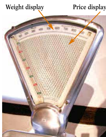
Fig. 6a Pendulum scales with variable weights and price indicating scale
