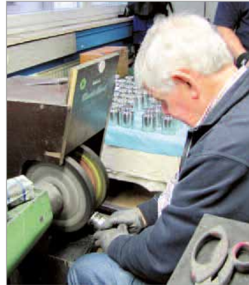
Figure 3: The weight blank for E_1/E_2 weights, for example (made with a small initial excess mass) is polished until the prescribed maximum permissible error on verification is obtained
