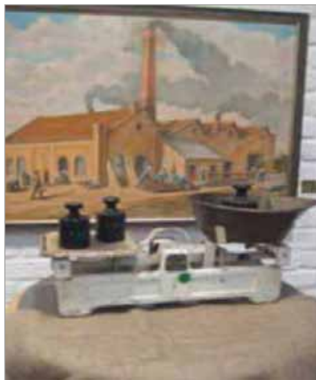
Fig. 2: Counter scales based on the principle of the equal-arm beam balance, around 1670
