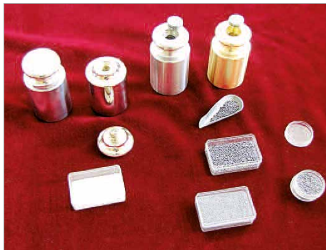
Figure 4: Weight blanks M_1-M_3 (right) with auxiliary equipment prior to final adjustment/verification. Fine-precision and commercial weights ( M_1, M_2, M_3 ) are usually manufactured with a slight underweight and equipped with an adjusting cavity. Small lead balls are filled into this cavity until the weight, including the fastening or the verification plate, complies with the prescribed maximum permissible error on verification
