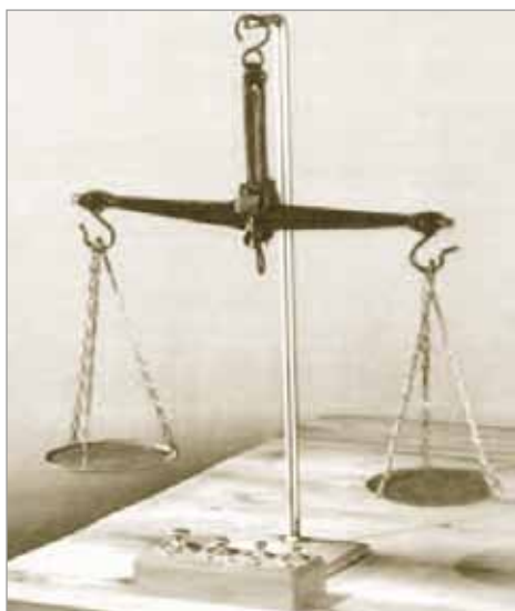
Fig. 1: Equal-arm beam balance, around 7000 BC
